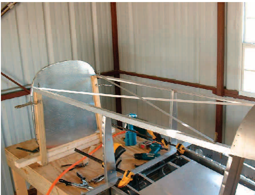
Front fuselage is squared and ready for assembly. Firewall is at left.
