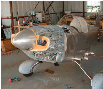
Cowling was made from wire cloth, which was then taped and fiber-glassed.
